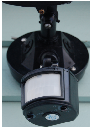
Figure 72. Garage door motion detectors are common applications of photoelectric sensors.
