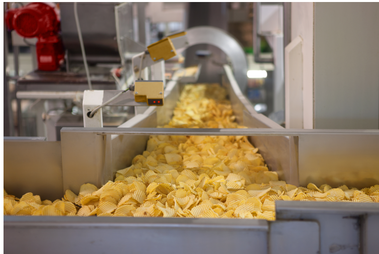
Figure 71. Diffuse light sensor used for the detection of potato chips on a belt conveyor.
