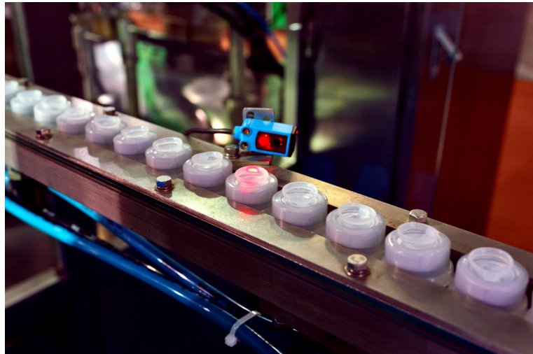
Figure 67. Diffuse light sensor used to detect the presence of caps on plastic containers in a production line.
